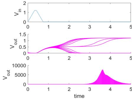
Fig. 5. Metastability analysis of fed back OR gate
