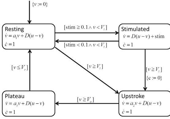
(a) Model of a single cardiac cell oscillator. The hybrid automaton has four locations corresponding to four phases of the oscillator. It has two continuous state variables  $v, c$  and two input variables  $u$  and  $stim$ . The remaining symbols represent constant parameters.
