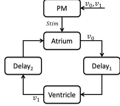
(b) Model of the whole heart-pacemaker interface. The model has 5 components. The Atrium and Ventricle are HIOA presented in Fig. 1a. PM is the pacemaker module.
