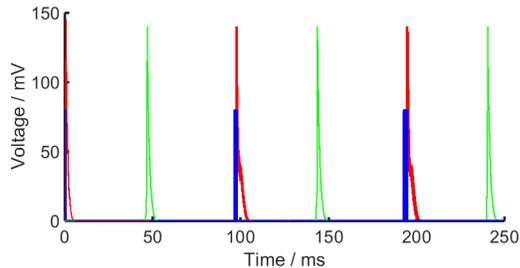
Fig. 3: Reach set of Example 1 with LR in the range [49, 51] and the two delays in ranges [45, 46], [51, 52]. The time duration property is satisfied in this case; however, we observe that, if we decrease LRI by 1, the atrium (red) will get excited twice in the last two cycles.
