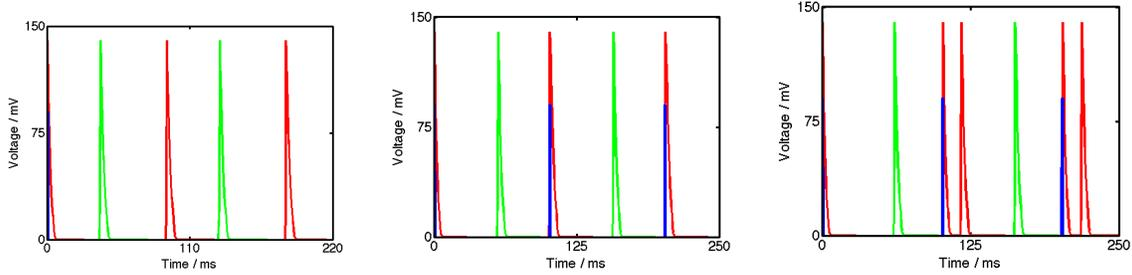
(a) The ventricle and atrium stimulate each other in turns with a proper rate. The pacemaker generates no impulse. (b) The pacemaker generates periodic impulses to keep the lower rate of the atrium. (c) The atrium is stimulated twice in a cycle, due to the pacemaker and the delayed pulse from the ventricle.
